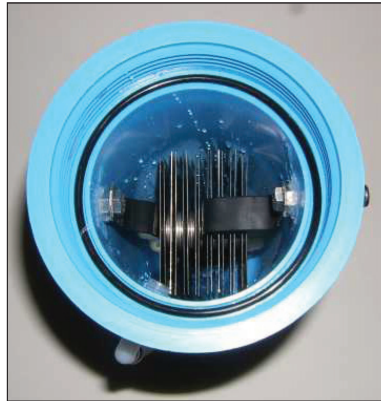
Inside are precision-spaced stainless steel plates hooked to electrical fittings. The "electrolyte" is common Sodium Hydroxide or drain cleaner! The electrolyte stays in solution and you rarely need to add to or replace it! Just add more water as needed!
