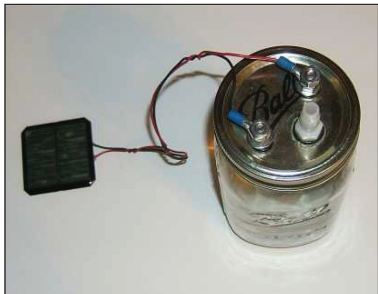
A "solar powered electrolyzer" built from a mason jar! It makes Hydrogen and Oxygen gas!
