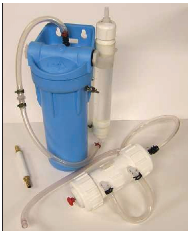
This is my most efficient "Hydrogen Electrolyzer." The blue electrolyzer, a safety "bubbler," a water/gas separator and a spark arrester. The blue housing is from a water filter.
